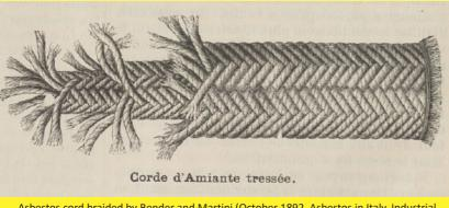
Asbestos cord braided by Bender and Martini (October 1892, Asbestos in Italy, Industrial Engineering)
