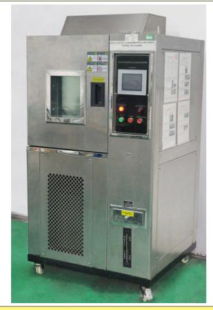
Climate chamber, with temperature adjustment range from -90 to + 150°C, relative humidity adjustment range 1 to 100%
