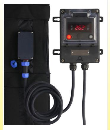
Electronic thermostat for NTC sensor. On-Off action, digital display. Remote wall mounting. Features a long temperature sensing probe for immersion in the liquid. Can be used in addition to surface temperature control, to end the reheating process when the core temperature of the liquid is reached. Attention: it cannot be used directly for the control of the heating, without it already exists a regulation of surface temperature, because it does not replace it.
