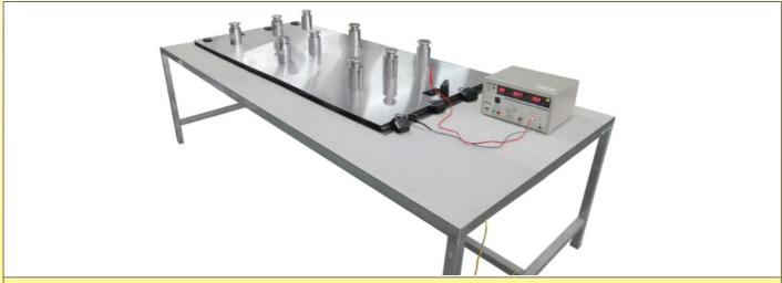
Measuring equipment for total current leakage at cold condition
