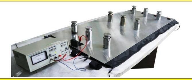
Device for measuring the insulation resistance.
