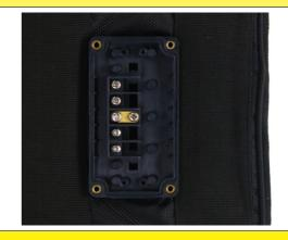
Simplified connection box, for fixed temperature jacket and blanket heaters. The surface temperature measurement is then performed by a bimetal limiter embedded in the heating wires network. Power supply "on" and heating "on" are displayed by 2 pilot lights. This control box version is not interchangeable with models of blanket or jacket heaters with built-in NTC sensor, intended for electronic control.
